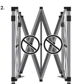
Be careful of the scissor sections of hardware as they are a pinching hazard.
