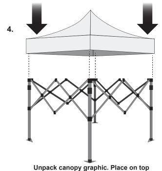
of frame. Align canopy corners with hardware corners and fasten together using the velcro.
