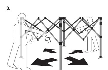
Standing across from each other, two people shoud use the center "V" of the hardware and lift up while stepping back. This will expand the frame. Stop when the frame is roughly 5 feet wide.
